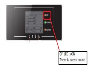
The AC side has leakage current to ground
